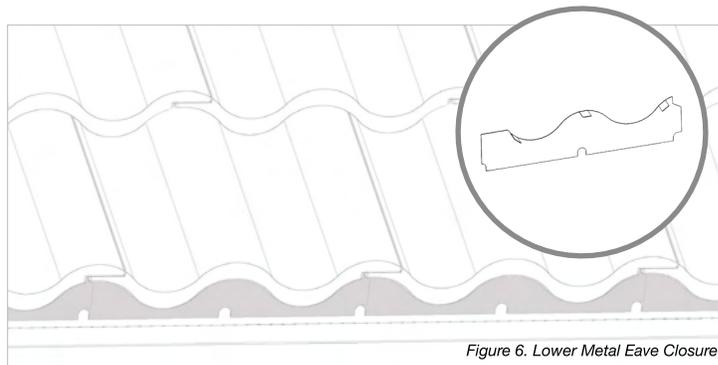
Quarrix Lower Metal Eave Closures, also commonly referred to as bird stop or bat stop, are individual painted steel pieces that snap into the Quarrix tiles located on any eave edge (the first row in any application). All Quarrix metal closures are G-90 galvanized steel, Kynar coated 24 gauge. Offered in compatible colors or black, these pressure fitted pieces fill what otherwise would be a visible void along the lower roof edge. The closure
