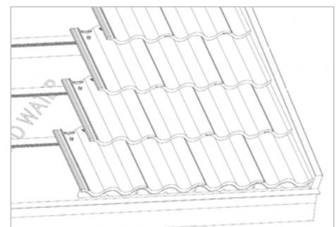
Figure 9. Field Tile Installation
