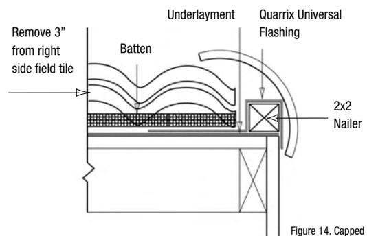
Figure 14. Capped Rake
