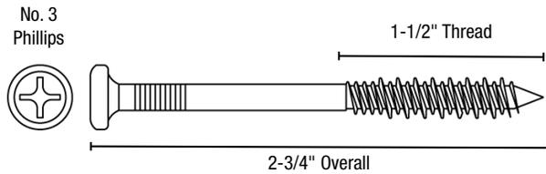
Quarrix Tile Fasteners are specially engineered and recommended for securing all Quarrix composite tile. Fasteners must penetrate the roof deck at least 3/4" (19.05 mm). Tile Fasteners are available in 1200-count pails and 100-count packs. Colors available: Black.
