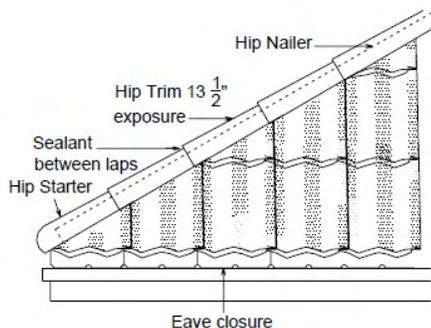
Miter cut Hip/ridge & Hip starter trim to fit. Add adhesive at the joint.
