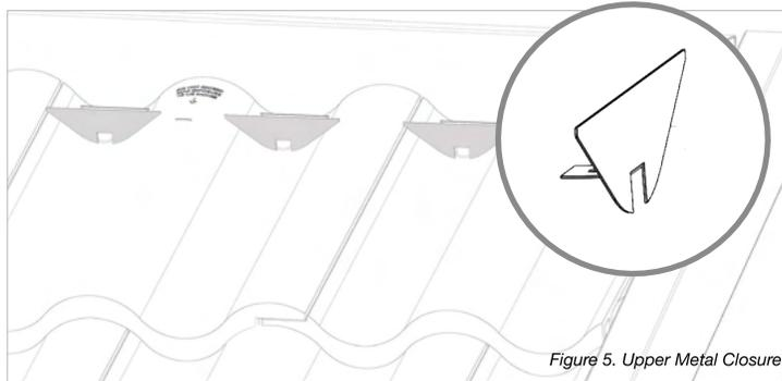
Quarrix Upper Metal Closures are designed for additional weather blocking in the top rows of tile installations. Typically, they are used in conjunction with pan flashing on roof to wall applications or in some ridge tile applications. If Quarrix Universal Flashing is used, upper metal closures are not required. Offered in compatible colors or black, these pieces attach to the tile as it is being fastened with the Quarrix Fastener. Two closures are needed for each tile. All
