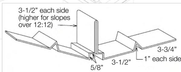
*\*Refer to Appendix C on pg. 26 for details on open and closed valley flashing. Generally speaking a closed valley will provide the most aesthetically pleasing valley configuration.*
