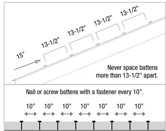
Figure 8. Batten Installation
