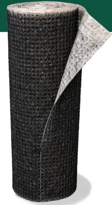
Quarrix ProTect Drain Mat creates a drainage plane and air cavity behind the cladding which helps prevent moisture damage to the walls and cladding. The ProTect Drain Mat also includes an extra 3” flap of the filter fabric that can be used for overlaps with other courses of the drainage mat or to create an insect screen at the top and bottom of the wall.
